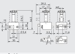
Description Cnomo 3/2 with bistable hand lever operator Code 88291B9
